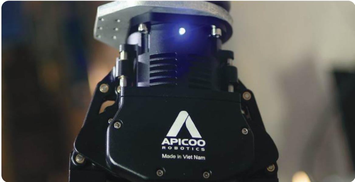
Figure 3.7 - The blue LED remains idle
